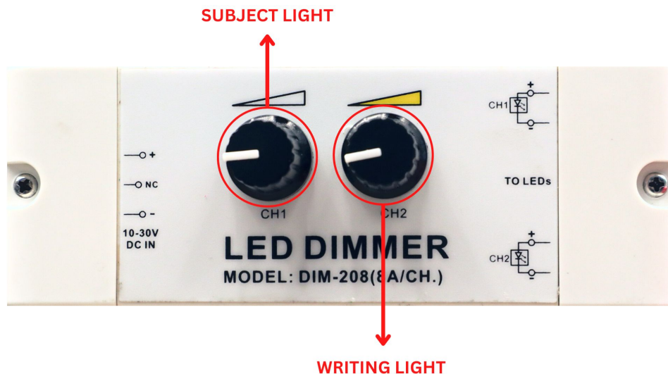
Fig. 1a. Brightness knobs on right side of board
