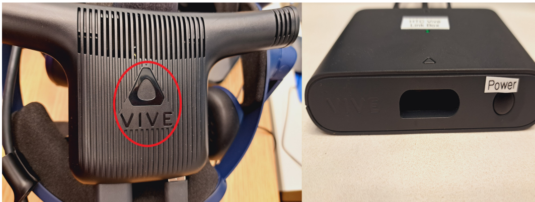
Fig. 1c. The triangular Vive Button (left) and the Link Box's Power button (right)
