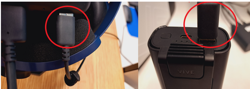
Fig. 1b. USB cable from the headset (left) to the battery (right)
