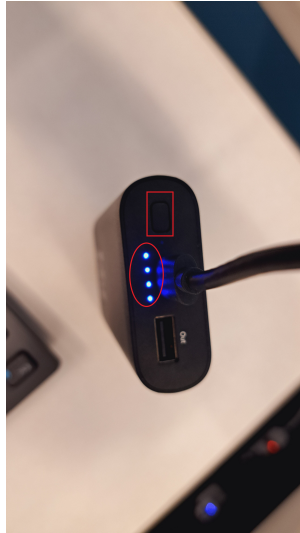
Fig. 1a. Battery with power button and four lights
